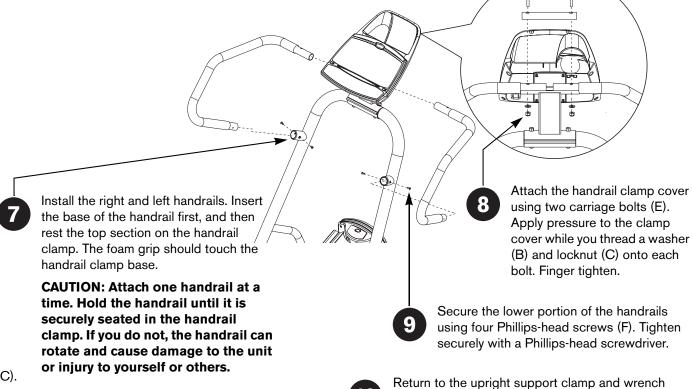
tighten the fasteners using a 9/16
